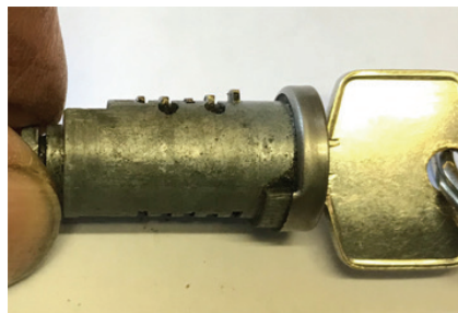
Picture 2 shows the key inserted, and the five 'pins' should all be flush with the surface to allow the cylinder rotate in the barrel.
