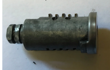
Picture 1 shows the cylinder without the key, and the five spring loaded 'pins' are extended and stop the cylinder rotating in the barrel.
