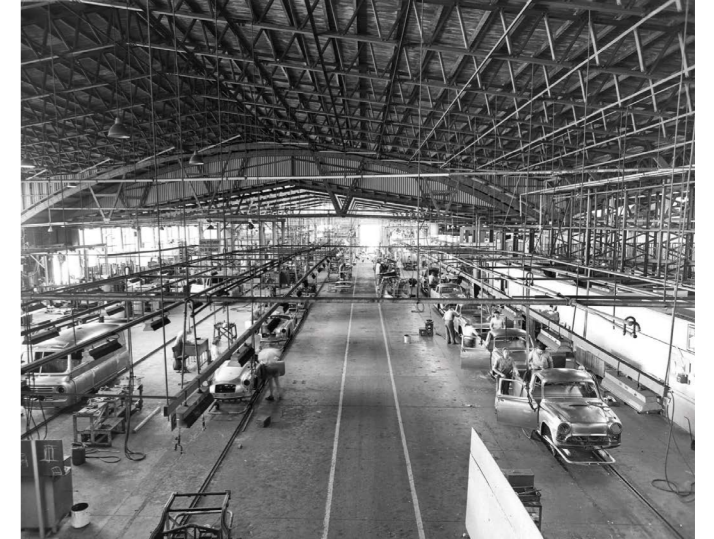
Pressed Metal Corporation factory, (spacious, light and airy compared to the dark cramped confines of the Abingdon factory). Showing L to R, lines constructing medium sized commercial vehicles, MGA line and "Ute" assembly. ("Ute" is short for utility vehicle. In American parlance, pick-up trucks) Note these vehicles are on temporary chassis called "skuks", moved along a track.
