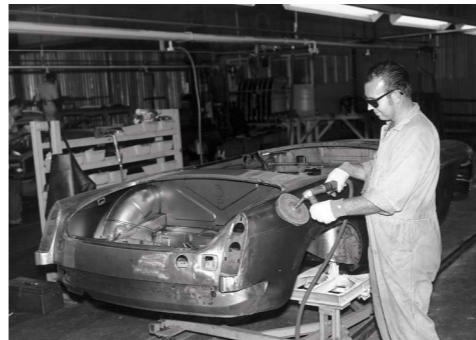
Finishing an MGB body shell. The leaded joint between the mudguards and the tonneau panel was problematic, with lead tending to bubble up in the paint ovens. Note the area of this joint has been sanded well back.
