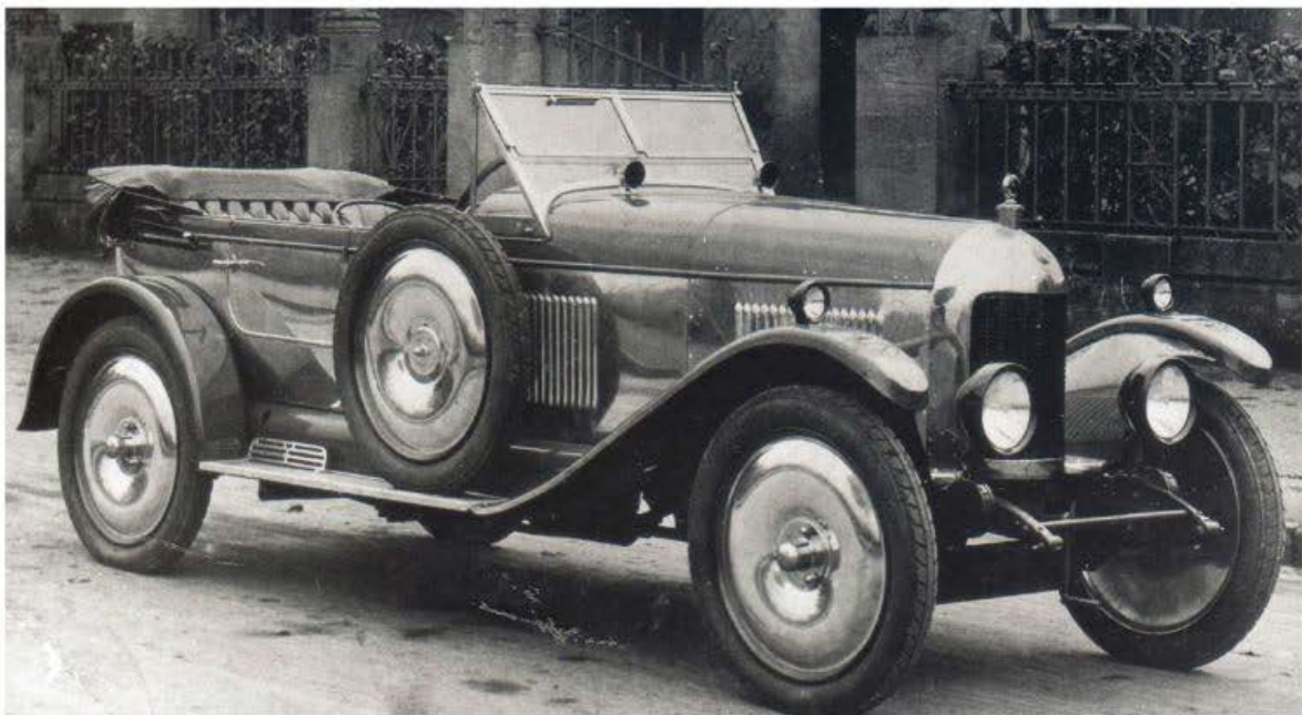
The 1925 model 14/28 Bullnose radiator MG Super Sports tourer – the nautical scuttle vents, the covers for the cast wheels and the triangular side-glasses for the opening windscreen were features of the Morris Garages bodywork.
