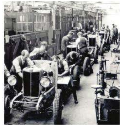
The small production line in early 1929 for assembling the first batch of MG 18/80 rolling chassis at MG's Edmund Road factory.
