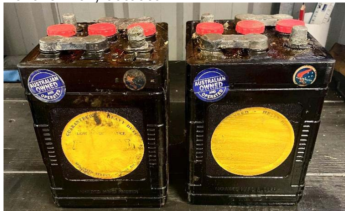
Above: two six volt Wet Cell batteries from an MGA.
