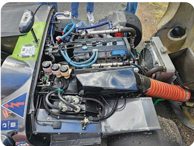
MG Midget engine bay 1800 cc K series 16 valve engine
